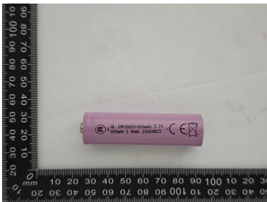
Figure 2 Side view of cell (IMR18650-800mAh)
